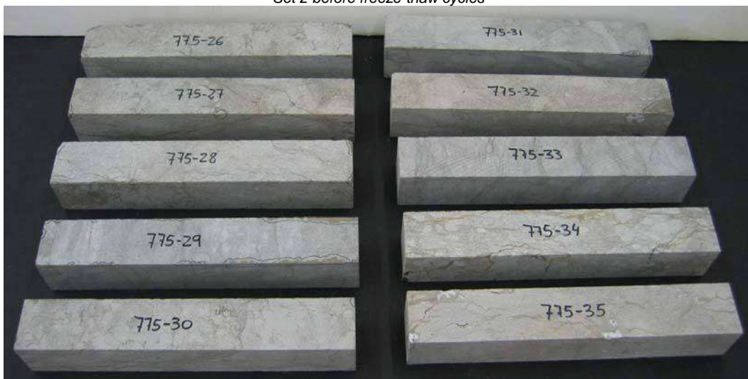
Lote 2 tras 56 ciclos de hielo–deshielo Set 2 after 56 freeze-thaw cycles
